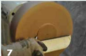
7 Turn a tenon on the body material.
