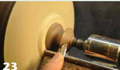
23 Final shape the top of the knob using the tailstock for support until the final cuts.
