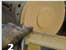
2 Turn a shallow tenon on the top of the lid.
