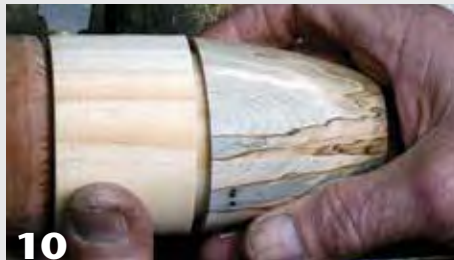
Use a softwood wasteblock to make a jam chuck. Transfer the inside diameter of the box to the wasteblock and form a tenon for a friction fit. This mounting can be reinforced with tape.
