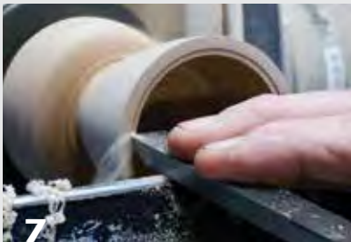
Use a square-end scraper to form a rabbet inside the box rim. This recess will accept the box lid.
