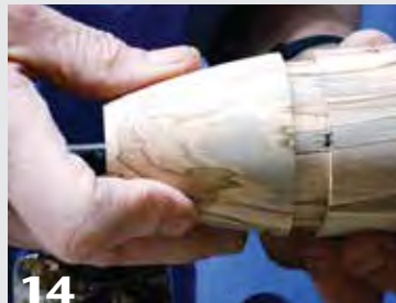
With the lid material mounted in the chuck and trued, use calipers to transfer the box's inside diameter to the lid. Then reduce the lid's diameter until you get a slightly snug fit in the box.
