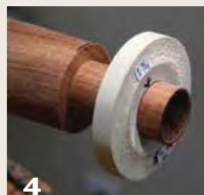
4 A simple gauge made by drilling the appropriate sized hole in scrap wood works well for checking your progress. Just slide the gauge over your workpiece (with the lathe off).
