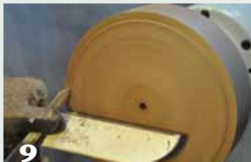
9 Transfer the inside diameter of the lid's lip to the body and turn a lip.
