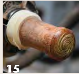
15 Jam chuck the outer box onto a waste block tenon to finish-turn the bottom.
