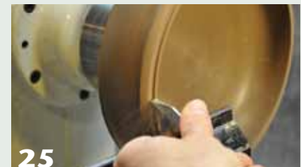
25 Adjust the lip of the body to achieve the final loose fit of the lid.
