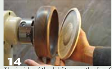
14 The inside of the lid fits over the lip of the body and for the next step, a jam fit is required.
