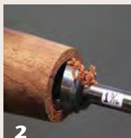
2 Use a 1 \frac{3}{16} " Forstner bit to create a visual reference for the wall thickness of the tube.
