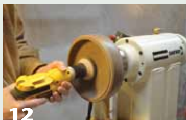
12 Sand the inside of the body.
