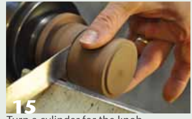
15 Turn a cylinder for the knob.
