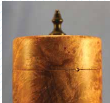
An unobtrusive pin affixed at the box/lid juncture registers the lid at the correct grain orientation.
