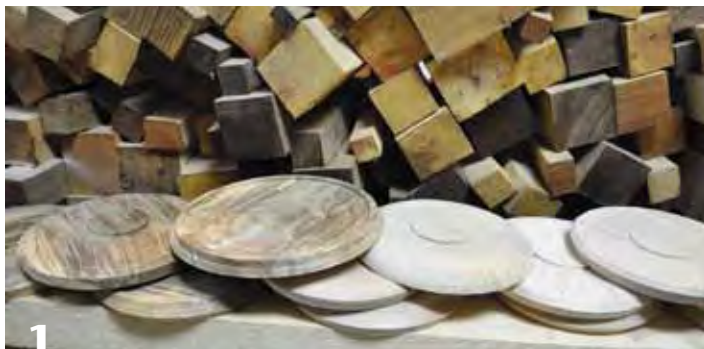
1 Several crossgrain box lids are rough turned for drying.
