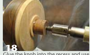
18 Glue the knob into the recess and use the tailstock as a clamp.
