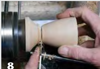
After gauging the box's inside depth, determine and mark the absolute bottom. Sand the box inside and out, then part it off the lathe.
