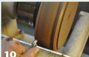
10 Shape the outside of the body and sand.
