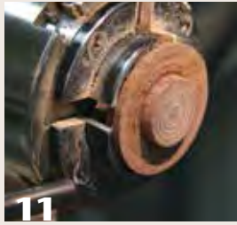
11 Form a bottom for the inner tube by creating a short tenon on the waste material, gluing the tube onto the tenon, and then parting the tube off. This creates a closed inner tube.
