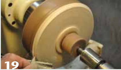
19 Shape and then sand the outside of the lid.
