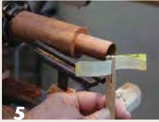
5 A safe way to sand inside a tube is to use a dowel to hold the abrasive.
