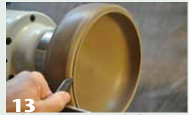
13 Make an adjustment to the lip to ensure a jam fit of the lid.
