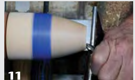
Using a sharp tool, gently shape the bottom so it is slightly convex. Sand the bottom.
