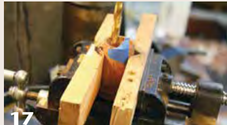
17 Drill a hole in the inner tube to accept a magnet.
