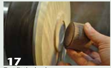
17 Test fit the knob.
