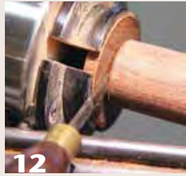
12 Glue the inner tube onto the tenon, and then part the tube off.
