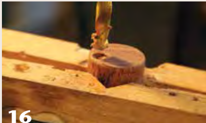
16 Drill holes near the edge of both tubes to accept recessed magnets, which provide a hidden method of holding the box closed.
