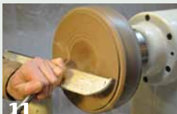
11 Hollow out and shape the inside of the body.
