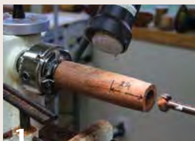
1 Drill into the purse box blank to form the inside walls of the inner tube.
