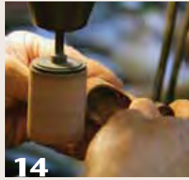
14 Carefully apply the inner tube to a drum sander to create the box's opening.
