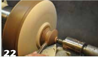
21 Shape the knob using either a round-nose scraper (l) or a small bowl gouge (r).
