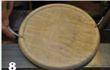
8 Measure the diameter of the lip inside the lid.
