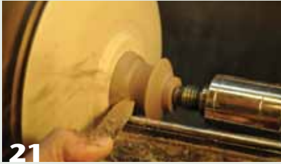
21 Shape the knob using either a round-nose scraper (l) or a small bowl gouge (r).
