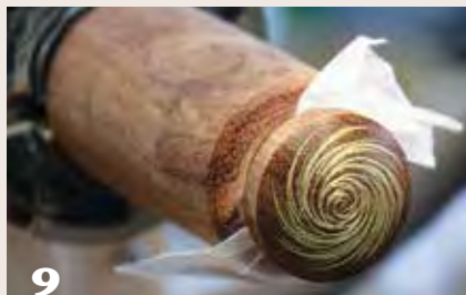
9 Use a hole drilled into the outer tube as a jam chuck to hold the inner tube for finish-turning its top. If the fit is too loose, add a layer of paper towel to take up the extra space.
