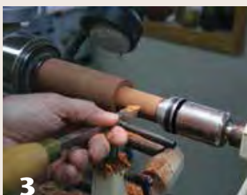
3 Carefully reduce the diameter of the inner tube.
