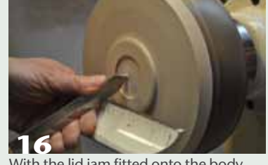
16 With the lid jam fitted onto the body, cut a recess into the center of the lid to receive the tenon on the knob cylinder.
