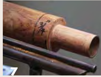
7 Indicate a section that will become the top of the inner tube. This is a good place for design elements such as beads, coves, or burn lines. 8
