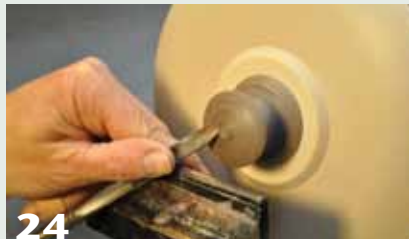
23 Final shape the top of the knob using the tailstock for support until the final cuts.
