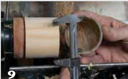
Use a softwood wasteblock to make a jam chuck. Transfer the inside diameter of the box to the wasteblock and form a tenon for a friction fit. This mounting can be reinforced with tape.
