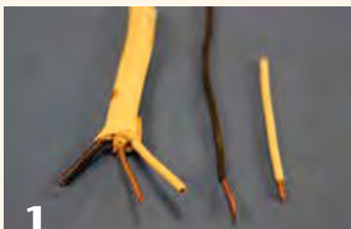
The copper core of 14/2-gauge electrical wire is a good choice of pin material.
